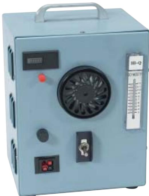
The CF-24B, FIXED SPEED, 12/24 VDC external battery operated field unit is ideal for remote site grab sampling. An elapsed, resettable timer (with independent 5 year battery) is incorporated into the unit housing to track exact sampling duration. The throughput flow rate is dependent upon the pressure drop across the filter media and the supplied voltage (12 or 24 volts DC). The CF-24B includes a 1 1/2" female straight pipe fitting which accepts the "CF" series filter holders.
