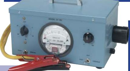
The CF-18V field unit operates on a single 12 volt automotive battery (not included). The two stage centrifugal fan pump motor is speed controlled by a rheostat which allows an operator to set a desired volumetric flow rate. An In-Line venturi allows for instantaneous flow measurement directly from an individually calibrated Magnehelic<sup>®</sup>. Continuous or 0-30 minute grab samples can be taken on a variety of "CF-Type" combination or paper only filter holders.
