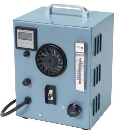
The CF970T-Series Air Samplers provide sampling time ranges from 0.01 seconds to 9999 Hours. Time ranges and operating modes are selected by front panel programming. There are eleven programmable time ranges and six programmable operating modes (i.e.: delay, interval, single shot,....). The programmable versatility makes the CF-970T ideal for grab and intermittent assay of particulate and radioiodine. Specify intended filter media type and desired flow ranges/units upon ordering.
