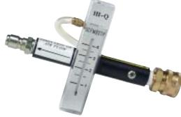
Precision machined venturi flow meter with NIST traceable flow calibration between the specified ranges described below. Each V-FLO-XX unit includes a 3/8" female quick disconnect on the inlet and a 3/8" male quick disconnect fitting on the outlet. For a complete description of HI-Q's Venturi Flow Meters, please see the "Air Flow Calibrators" section of this catalog.
